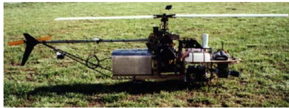
Figure 1 - ASRT vehicle weighed approximately 35 pounds
