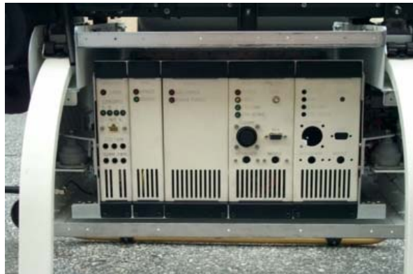
Figure 7 - Vibration isolated avionics module rack, from left to right: data link module, GPS module, computer module #1 (flight computer), computer module #2 (auxiliary)
