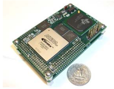
Figure 13 – FCS20 miniature autopilot performs navigation, guidance, and adaptive control for small UAVs.
