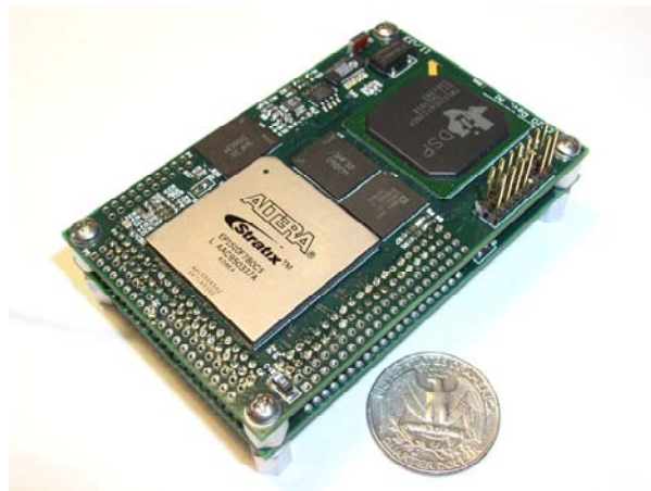
Figure 1 A credit card-sized board designed with the processing power and flexibility required for deployment in highly-capable small UAVs.
