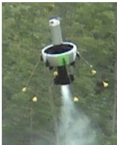
Figure 7 HeliSpy 11 inch ducted-fan UAV, weighs between five and seven pounds
