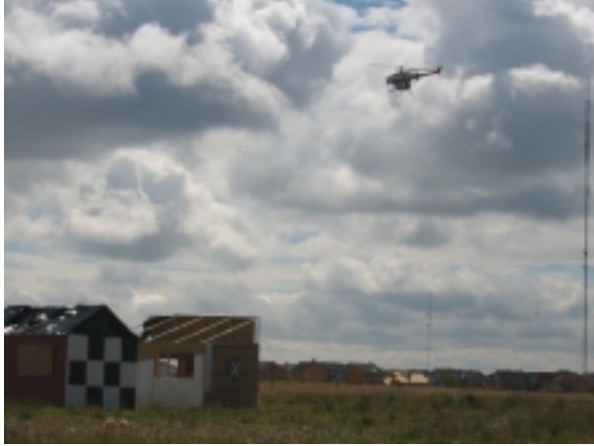
Figure 12 – GTMax automatically locates buildings in search area during 2002 International Aerial Robotics Competition; here it is automatically looking for openings into the buildings
