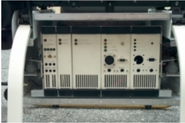
Figure 2- Vibration isolated avionics module rack, from left to right: data link module, GPS module, computer module #1 (flight computer), computer module #2 (auxiliary)
