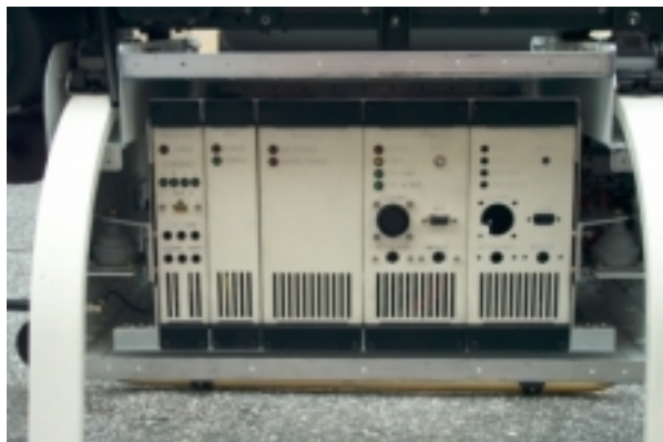
Figure 2- Vibration Isolated Avionics Module Rack
