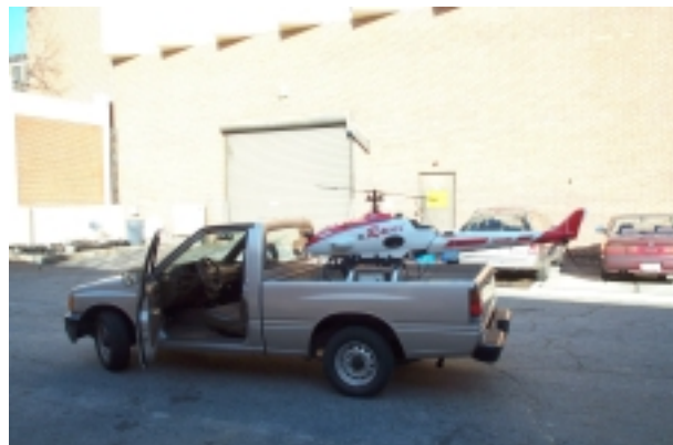
Figure 9 – Truck testing of Navigation System
