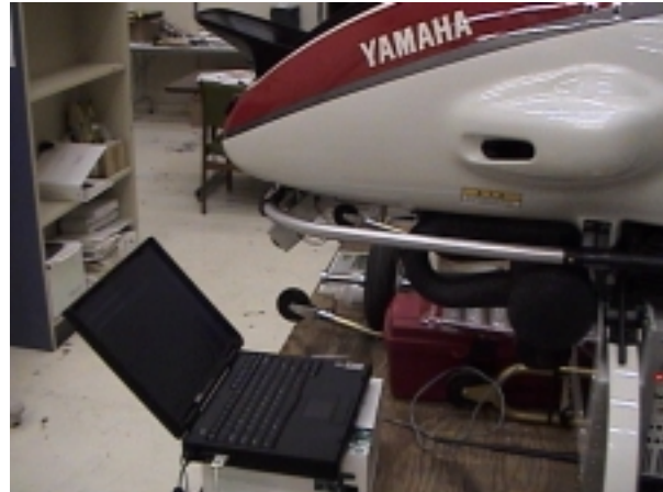
Figure 12 – One of the Image Processing Test Configurations, Simulated Images are Being Shown to the GTMax Onboard Camera
