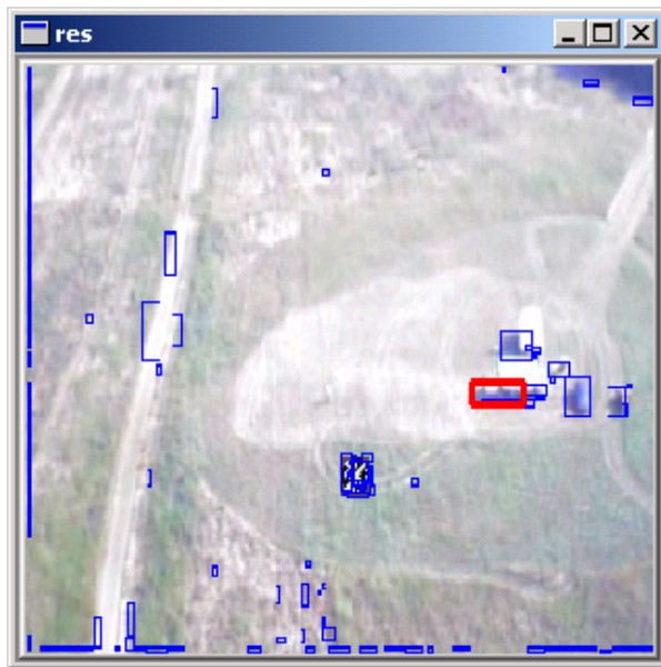
Figure 11 – Onboard Single Image After Processing, Red box Indicates a Correctly Located Building
